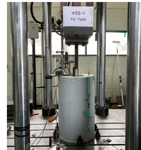
(b) Anchorage Test Specimen
