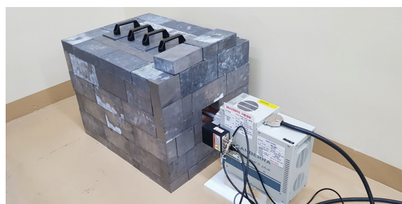
Fig. 2. HPGe gamma-ray detection system for measurement of delayed gamma-ray from the ^{167}\text{Yb} radioactive isotope sample.
