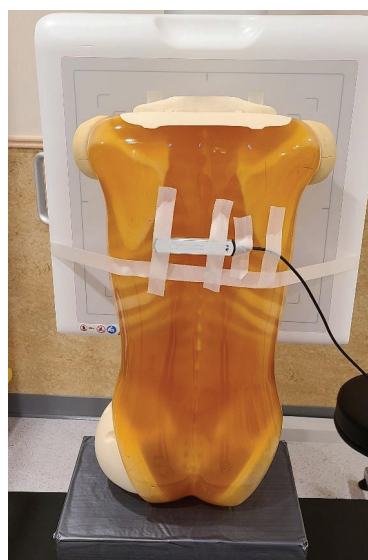
Fig. 2. PBU-50 is attached transverse to the dosimeter in position 7th~8th to the thoracic spine.
