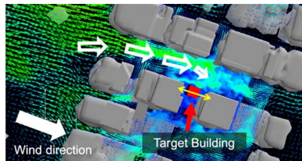
Figure 18. Flow visualization. (wind direction of 270°)
