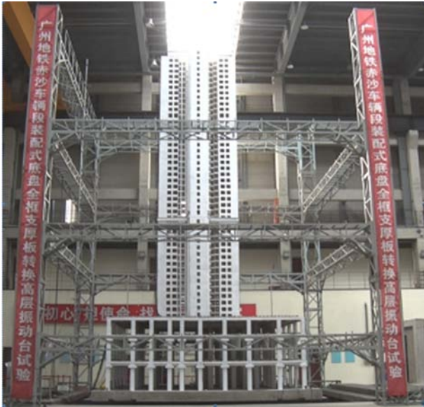
Figure 9. 1/10 scaled physical model for shaking table tests.
