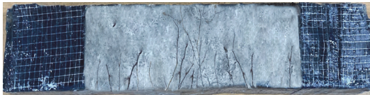
Fig. 14 Cracking picture of specimen strengthened with carbon fiber sheet and end anchorage
