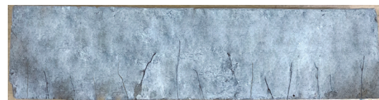
Fig. 10 Cracking picture of reference specimen
