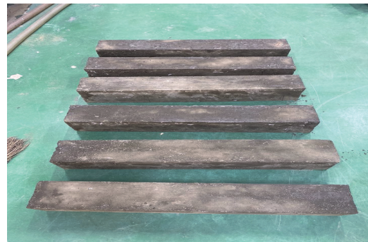
Fig. 4 Test specimens after removal of forms
