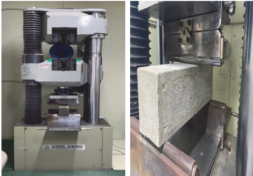
Fig. 6 Flexural strength test
