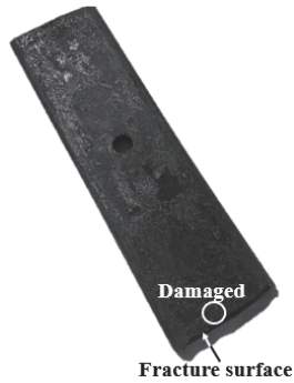
Fig. 2 Fractured appearance of leaf spring
