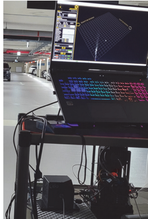
Fig. 9 Distance measuring test of low optical power LiDAR
