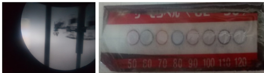
Fig. 6. Measured the surface temperature using thremo-label during ta-C coating.
