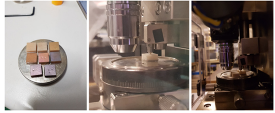
Fig. 3. Nano-indentation test of ta-C coating on polymer substrate.
