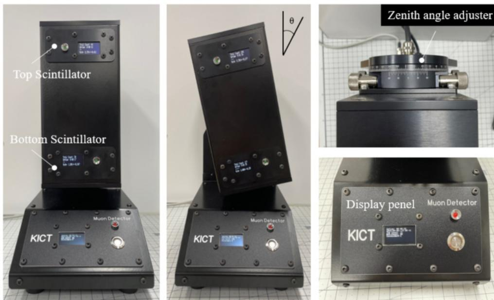
Fig. 3. Photo and configuration of the muon detector prototype
