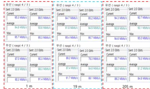
Fig. 15 Communication speed performance evaluation of wired/wireless communication repeater
