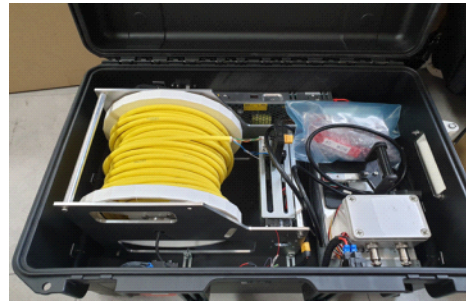
Fig. 11 External power supply system
