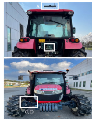
Fig. 4 Agricultural tractor with modular steering control system(A : RTK-GPS, B : IMU, C : Hydraulic valve, D : Wheel angle sensor)
