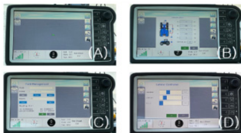
Fig. 2 HMI (A : Main display, B : Vehicle specification setting, C : Field management, D : Lateral controller)
