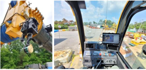
Fig. 8 Sensor Setup to 250ton Crane (left), User Interface in Cabin (right)
