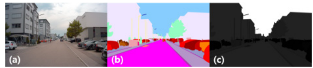
Fig. 4 (a) Raw image, (b) Original labeling of A2D2 dataset, (c) Preprocessed labeling of A2D2 dataset
