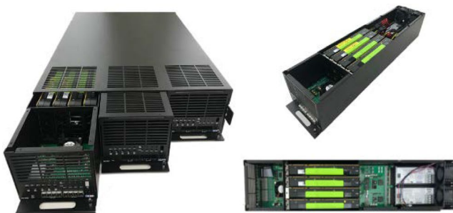
FIGURE 4 HD-PEX, a proprietary high-density multi-GPU hardware subsystem
