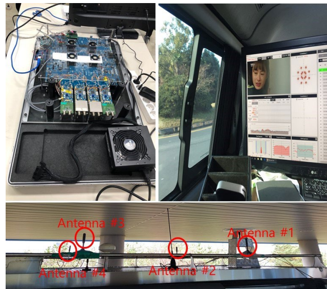
FIGURE 8 Experiment environment description: Prototype MR implementation (upper-left), real-time signal analysis within the test vehicle (upper-right), and antenna installation at the test vehicle (bottom)
