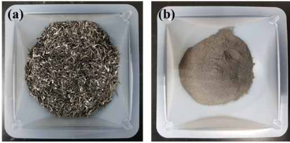
Fig. 3 Photograph of Ta scrap (a) Raw scrap, (b) Hydride powder after milling
