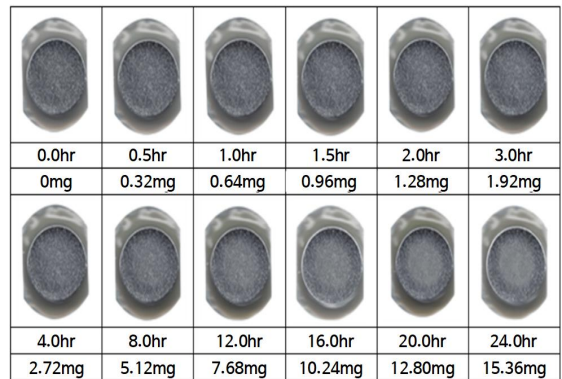
(a) Corrosion amount shape of 'C'
