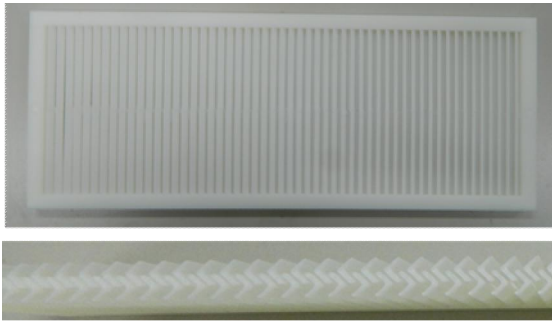
Fig. 6 Type 6 filter created with 3D printer
