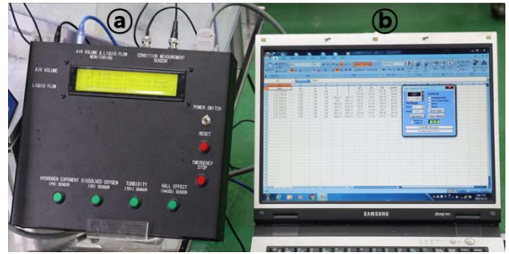
Fig. 4 Photograph of real-time monitoring device installation and operation
