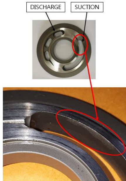
Fig. 3 Cavitation of a valve plate
