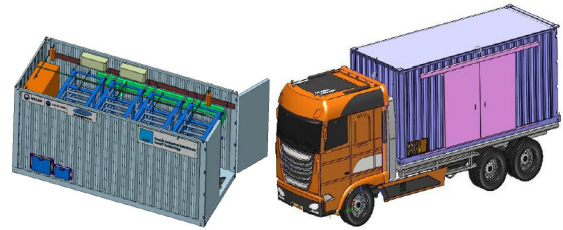
Fig. 4. Concept of removable battery truck.
