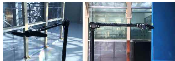
Fig. 7 Installing of the Propeller Test Stand
