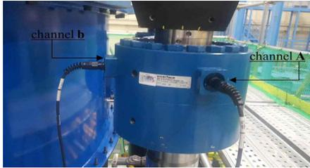
Fig. 11 Channel A and b of Load Cell
