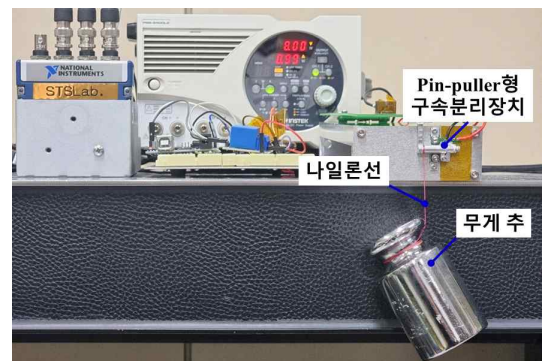
Fig. 10 Static Loading Test of Pin-puller Mechanism
