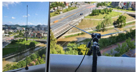
Fig. 3 Installed Whip Antenna / Dipole Antenna
