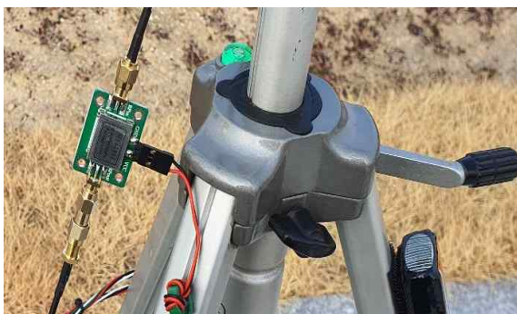
Fig. 15 Installed External LNA
