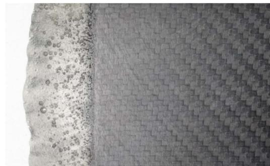
**Fig. 13.** Resin squeeze out effect
