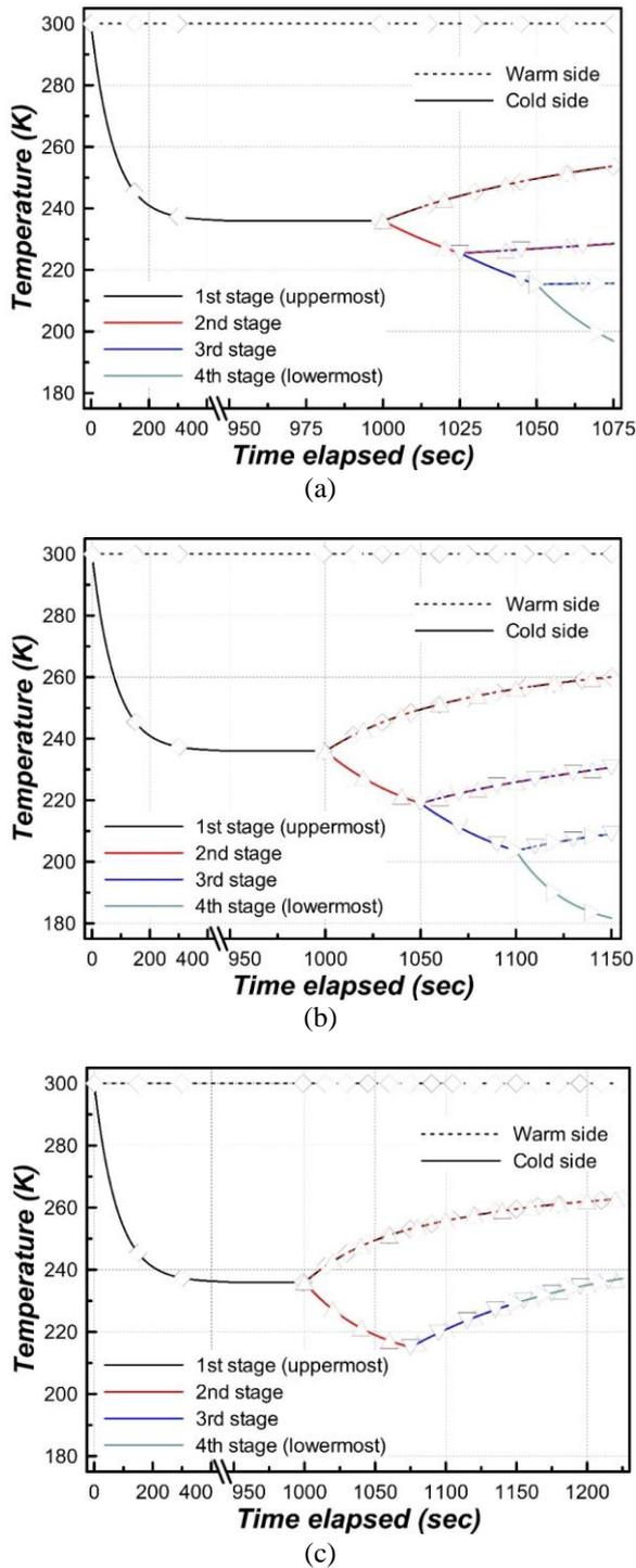
Fig. 5. Temperature variation during transient operations; holding duration for (a) 25 seconds, (b) 50 seconds and (c) 75 seconds.
