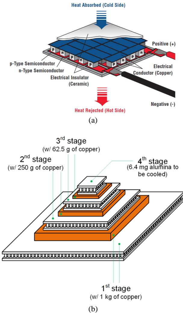
Fig. 1. Schematic diagrams of (a) a thermoelectric module and (b) multistage TEC with thermal masses.
