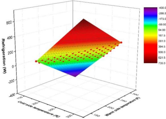
Fig. 3. Curve fitting for refrigeration; negative values are not meaningful.
