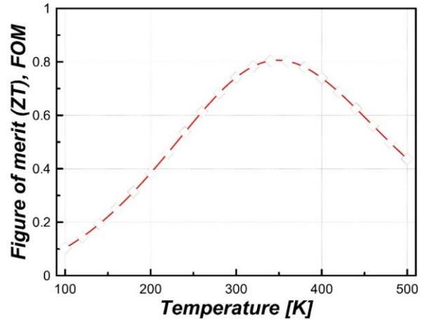
Fig. 2. Figure of merit of bismuth telluride ( $\text{Bi}_2\text{Te}_3$ ).
