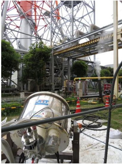
Fig. 4. Solenoidal superconducting magnet in the field experiment.
