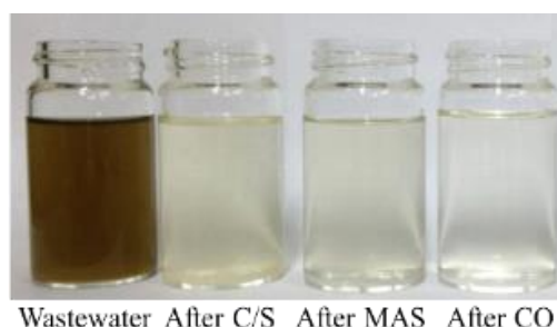
Fig. 3. Photograph of the farm wastewater, treated water after C/S, treated water after MAS and treated water after CO.
