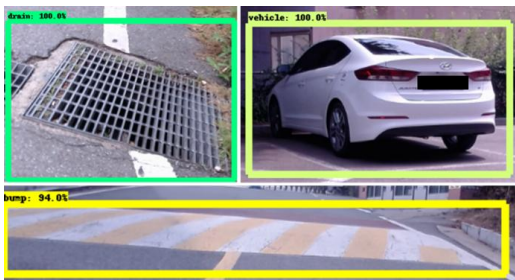
Fig. 7. Obstacle detection test examples: drain cover, vehicle and bump
