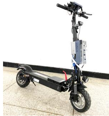
Fig. 6. Electric kickboard with automatic emergency braking system and safe starting system
