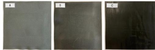
Fig. 2. Manufactured tungsten shielding sheet appearance. (a) tungsten oxide shielding sheet, (b) tungsten carbide shielding sheet, (c) pure tungsten shielding sheet
