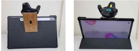
[Fig. 2] Mobile augmented visualization system hardware configuration
