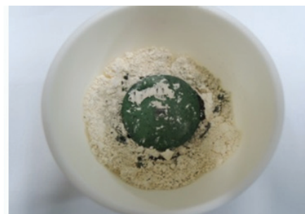
Fig. 1. \text{YBa}_2\text{Cu}_3\text{O}_{7-y} superconducting bulk with \text{Gd}_2\text{O}_3 powder heat diffusion.
