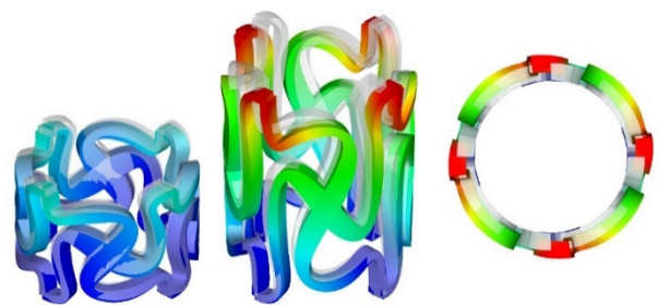
Fig. 11 Parametric study on height of cylinder (a) 30mm, (b) 60mm, (c) top view of 60mm model
