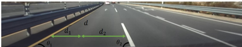
Right Warning and Departure Status
