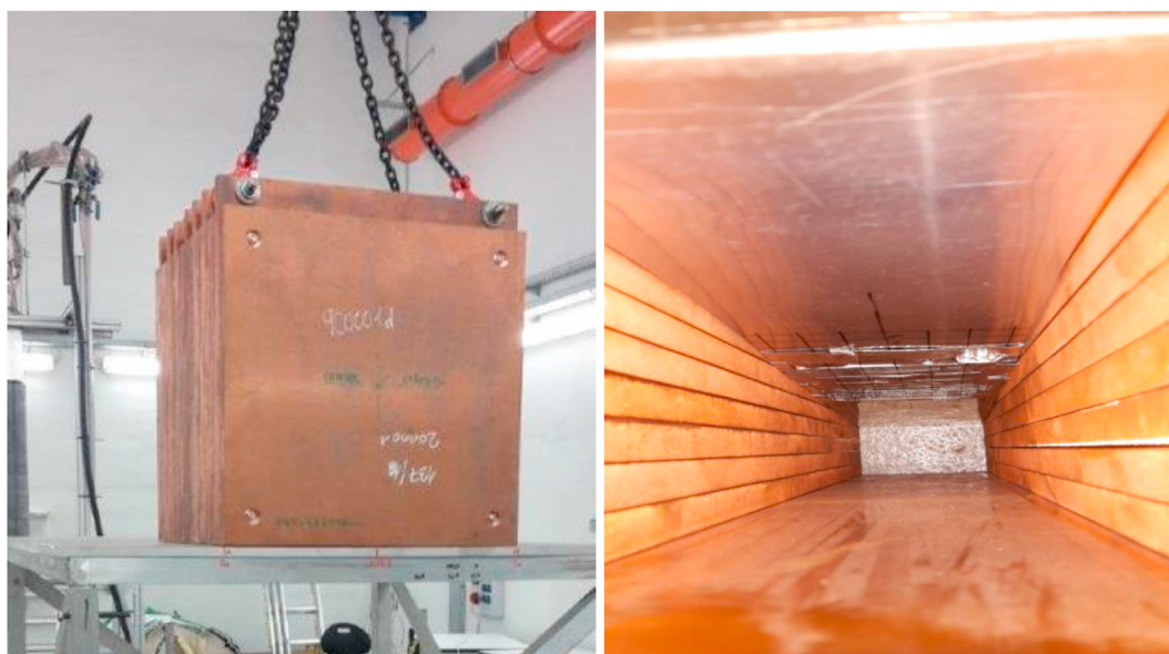
Fig. 2. Left: Copper block was used for the experiment. Right: activation foils holder made of aluminium.
