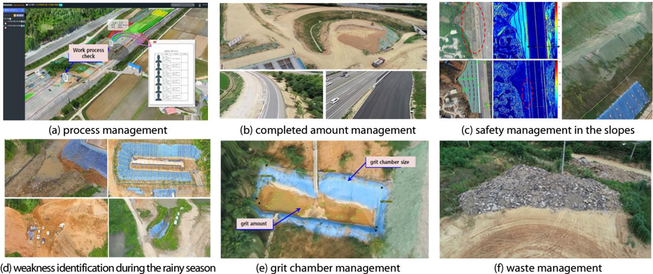
Fig. 6. Drone application Result of Detailed Construction Management Work Type (2)
