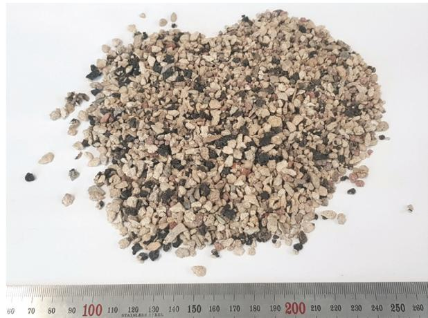
Fig. 1. Recycled aggregates used
