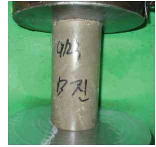
Fig. 6. Compressive strength test
