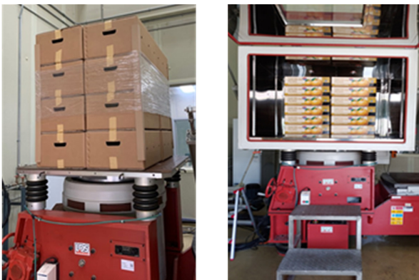
Fig. 3. Vibration simulation test of unit load system for pears.
