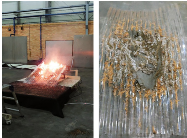
Fig. 7. Forest fire firebrand test results for polycarbonate sheet
