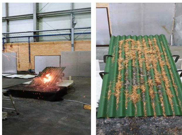
Fig. 8. Forest fire firebrand test results for asphalt shingles
