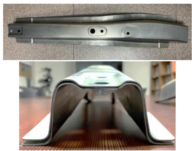
Fig. 11 Stamping result of front side rear lower member
