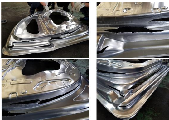
Fig. 3 Formability problem of AA6016 hot stamping (Heating temp. : 530 °C)
