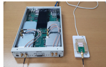
Fig. 1 Implemented hardware testbed for RF fingerprinting.
