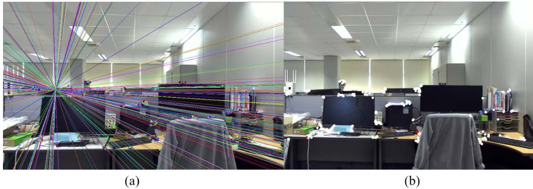
Fig. 2. The example of outlier removal process with epipolar geometry (a) epipolar line example (b) outlier detected by epipolar geometry. Red dots are considered as outlier.
