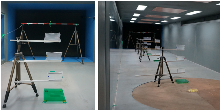
Fig. 3 Scenes of spray drift experiment in wind tunnel
