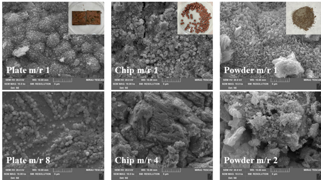
Figure 5. FE-SEM morphology of cementation products by Fe to Cu molar ratio conditions and iron samples.
