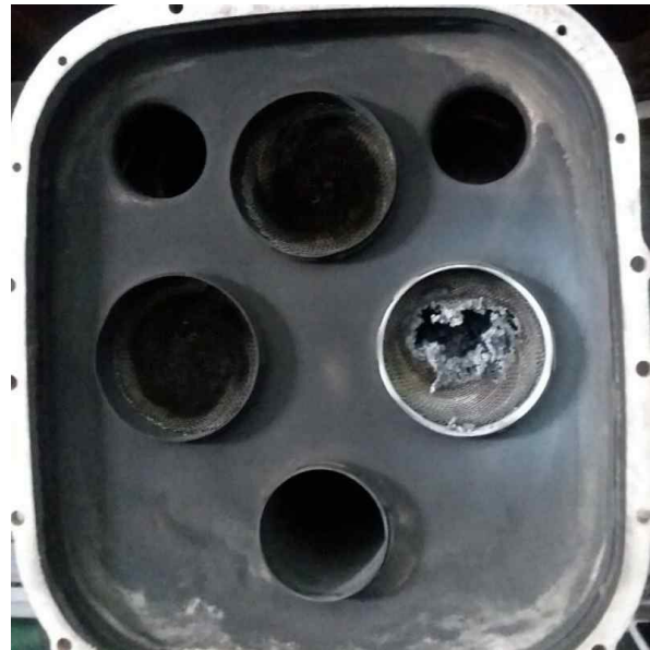
Fig. 10 2011 Mecha truck DPF melting
