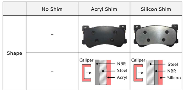
Fig. 10 Shapes of damping shim
